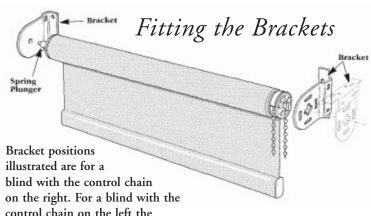
control chain on the left the brackets should be at the opposite ends. Brackets can be fixed to any flat surface above, behind or to the side of the blind. They must be level to ensure the smooth operation of the blind. Check that the rolled up fabric will not touch any surface. To calculate the spacing between the brackets add 32mm (1 1/4") to the width of the blind fabric. Fix the brackets so that the outsides of the brackets
