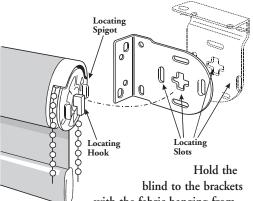
with the fabric hanging from the back of the blind. Fit the spring plunger into its bracket. Push the blind into this bracket, depressing the plunger. With the locating hook pointing downwards place the hook into the vertical part of the '+' shaped hole in the bracket. Allow the hook to drop downwards so that it locks into place in the bracket.
