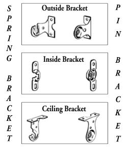
Spring end (flat pin) always goes to the left side and the round or pin end to the right side.
